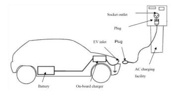
In mode 1, 2 and 3 the charging takes place through the converter in the vehicle (AC from the charging station to DC in the vehicle battery) and the charging process is being controlled by the vehicle. The capacity of the converter determines how much of the available charging capacity of the charging station can be utilized.
